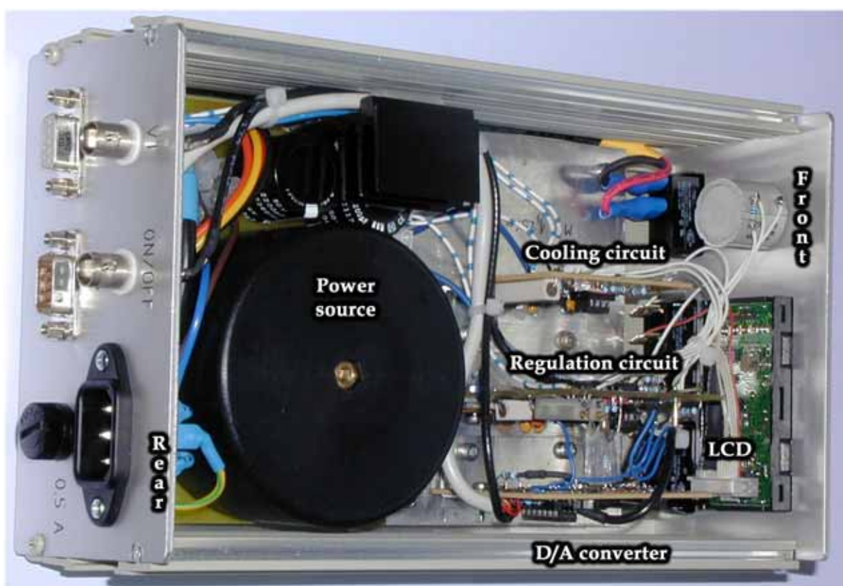
Fig. 93. Thermostat hardware (top view)
