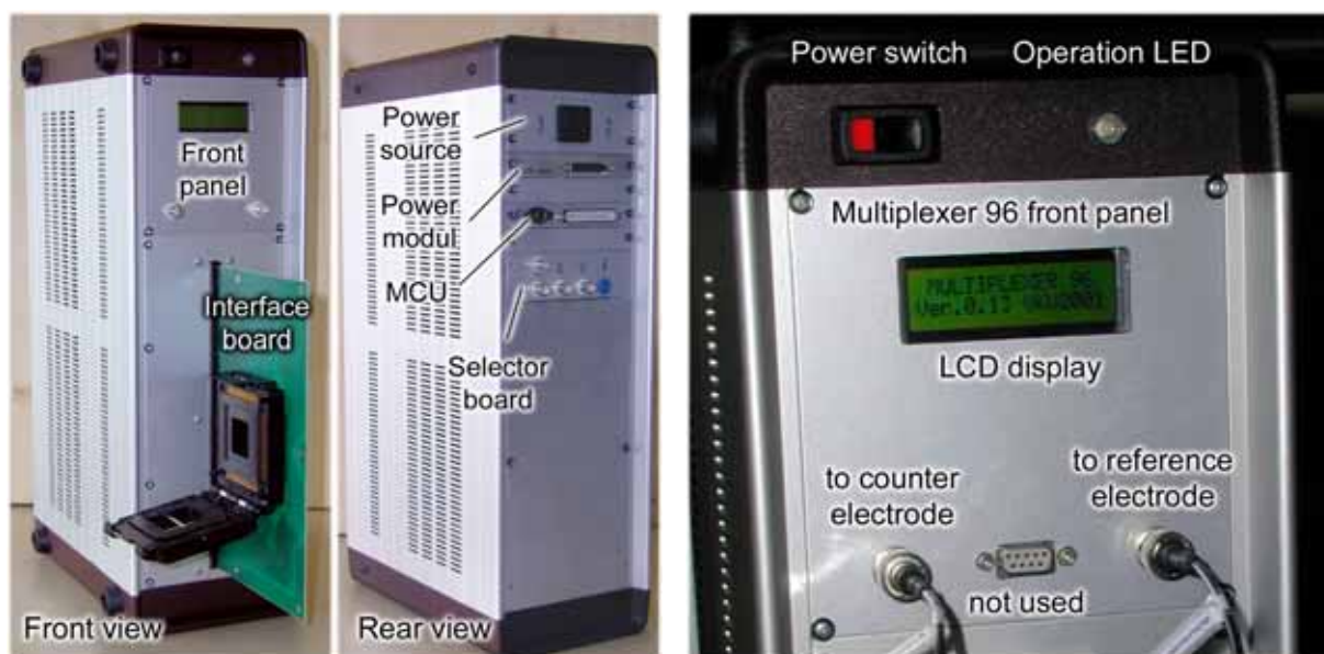
Fig. 32. Multiplexer 96, rear and front view (left), detail of MX96 front panel (right)
