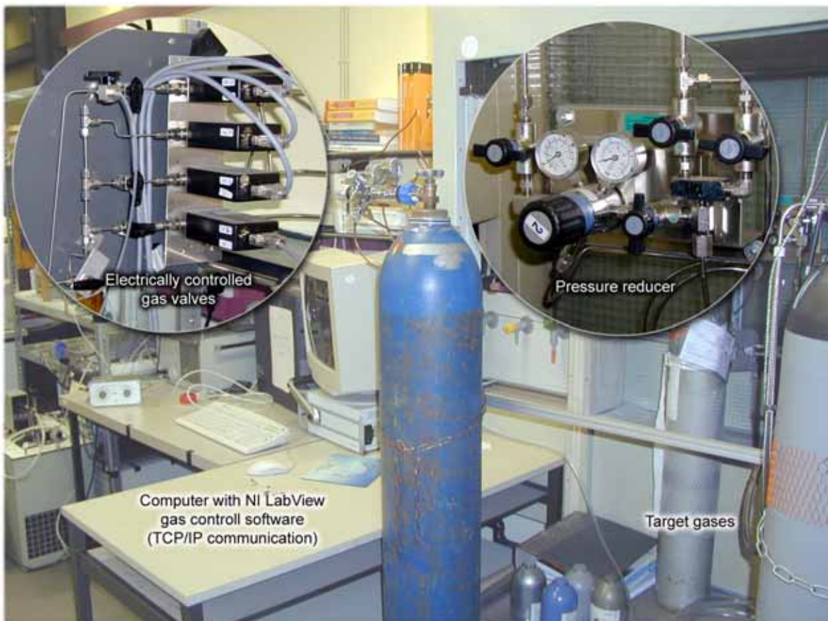
Fig. 67. Practical realization of the gas flow system
