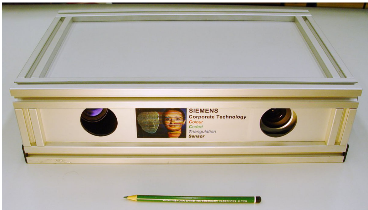
Figure 48: Exemplary prototype system based on the coded light step of the proposed ranging approach. A similar set-up – that is one without the housing to allow an arbitrary choice of the baseline and the integration of a second camera – is used for the experiments of this section. The dimensions of the portable system shown are about 0.45 m x 0.25 m x 0.1 m.
