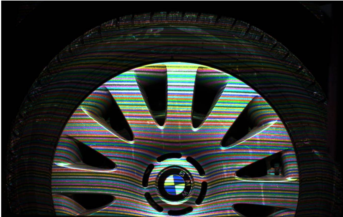
Figure 64: Image of a car wheel illuminated by the projection pattern.
