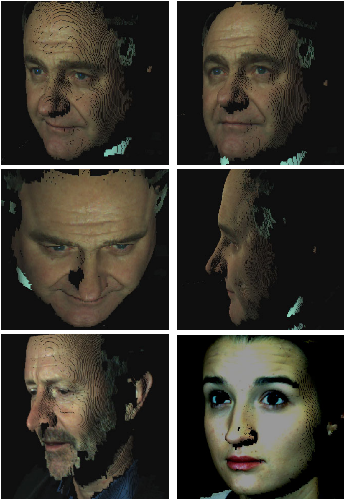
Figure 59: Several point clouds of human faces corresponding to frontal range images. The top four views are all generated from the same range image.
