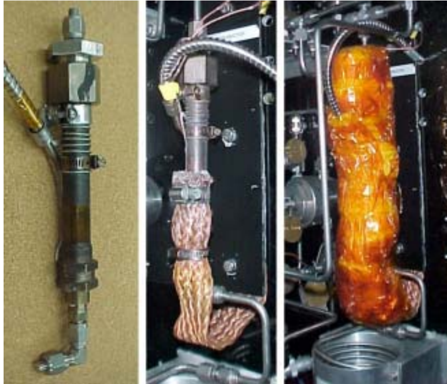
Figure 4-7: Sabatier Reactor, with Copper Strap, with Insulation
