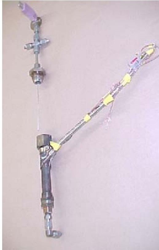
Figure 6-2: Reactor Top with Thermocouple
