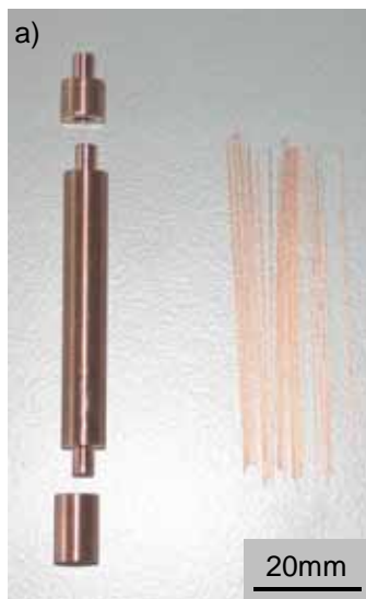
Figure 2.11.a) Coated fibres to be consolidated in the copper capsule; b) HIP parameters
