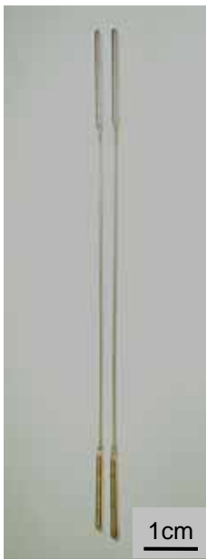
Figure 3.48. Coated fibres prepared for tensile test
