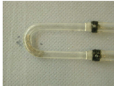
Abb.13: Stent I: A Jomed Self-X-Stent, 6mm in diameter and 32 mm in length, was placed from 0-90° (elbow start to apex)
