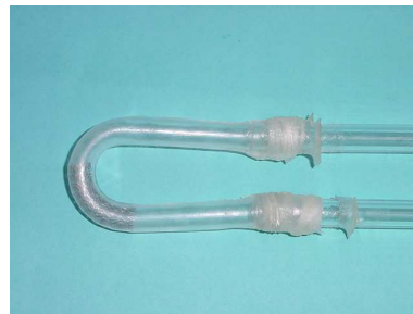
Abb.15: Stent III: A Jomed Self-X-Stent, 8mm in diameter 32mm in length, was placed from 0-90° (elbow start to apex)
