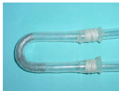
Abb.16: Stent IV: A Jomed Self-X-Stent, 8mm in diameter 64mm in length, was placed from ca. 0-180°. (elbow start to elbow end).
