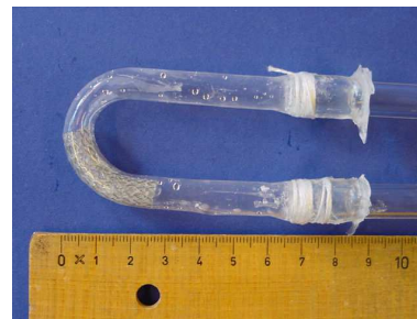
Abb.18: Stent VI: A Jomed Covered Stent, 8mm in diameter and 32mm in length, was placed from 0-90° (elbow start to apex)
