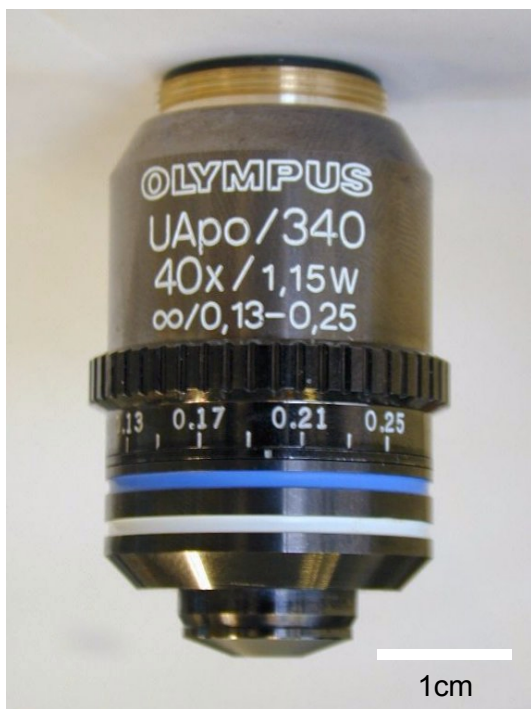
Fig 5.3 High aperture water objective. With 40x magnification, 1.15 numerical aperture without plane correction and a built-in cover slip this objective offers a maximum excitation and emission efficiency. The working distance is 260 \mu m. The chip design was heavily influenced by the large size of the objective.
