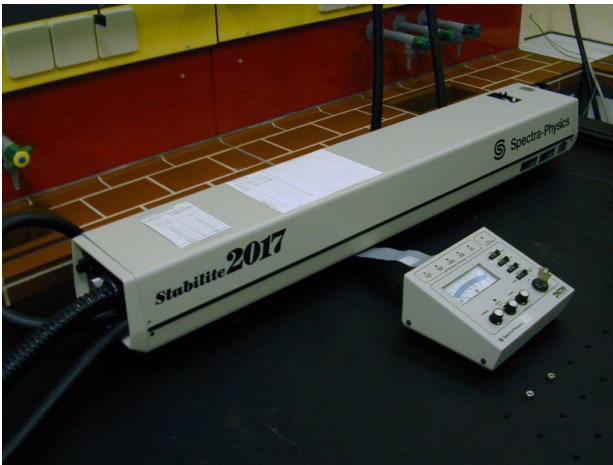
Fig 5.4 Argon ion laser used for the confocal microscope (left). It can be switched to different wavelengths and couples to a single mode fibre (right)
