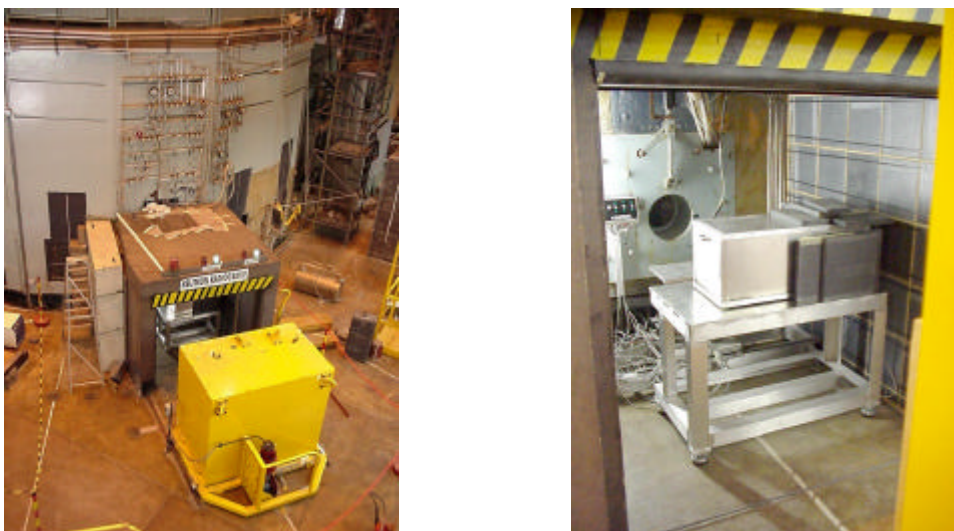
Figure 6.10: A view on the thermal radiography station at SAFARI-1. The location of the setup in respect to the reactor (left). A look at the experimental bunker (right)
