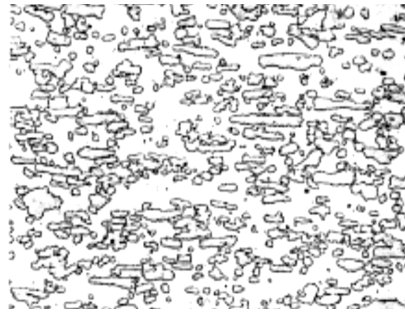
Figure 7.5: A slice image of a boron alloyed steel sample taken by SEM in a 3.75 mm line.
