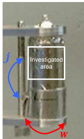
Figure 4.10: The used MnSi polycrystal in the topography experiment. The investigated area is marked in the photo.
