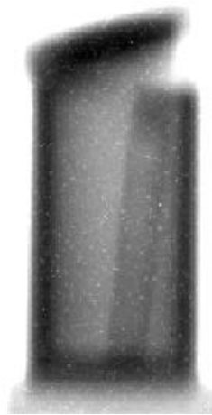
Fig. 8.10: Shielding container (lead) with slightly opened lid containing a cylindrical europium source.
