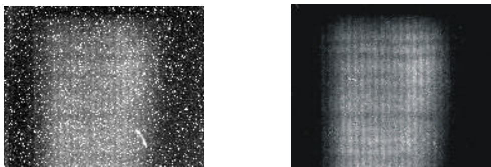
Figure 4.7 At a defined reflection position a number of projection images were taken (left). The final topography image (right) was obtained as a summation of the corresponding projection images after their correction for white spots and dark current.
