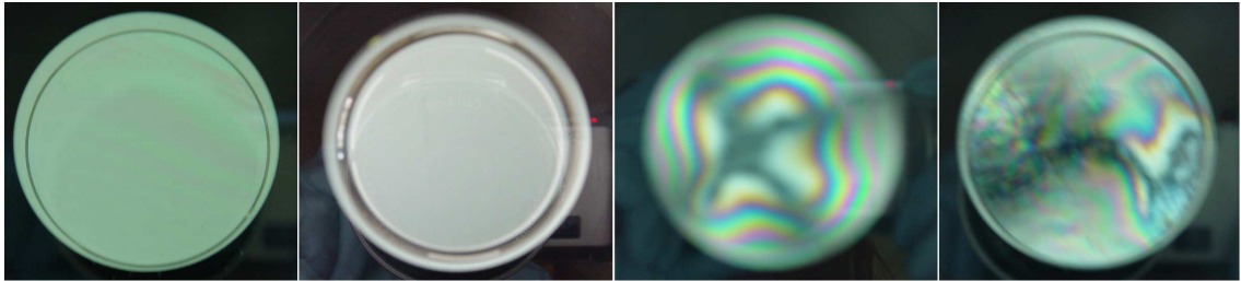
Figure 5.30: Photoelasticity photos of four \text{CaWO}_4 crystals using white light. From left to right, photos of Boris (Ukrainian), Rita (Russian), K08 (Karat), and Ch08 (Chinese) are shown.
