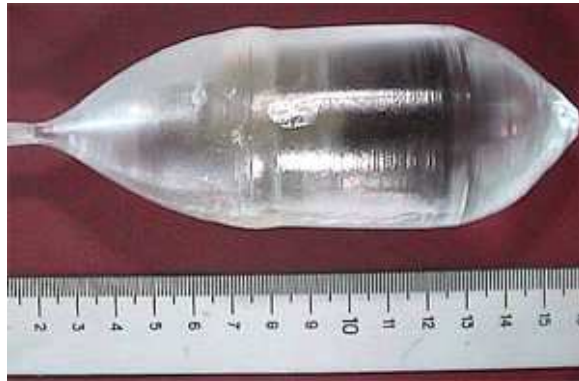
Figure 5.1: \text{CaWO}_4 , ingot as grown.
