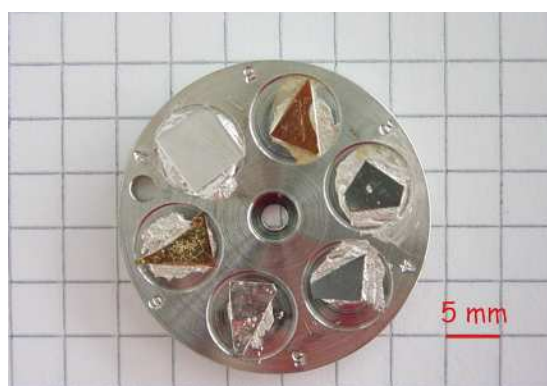
Figure 4.5: Target holder with six different materials.
