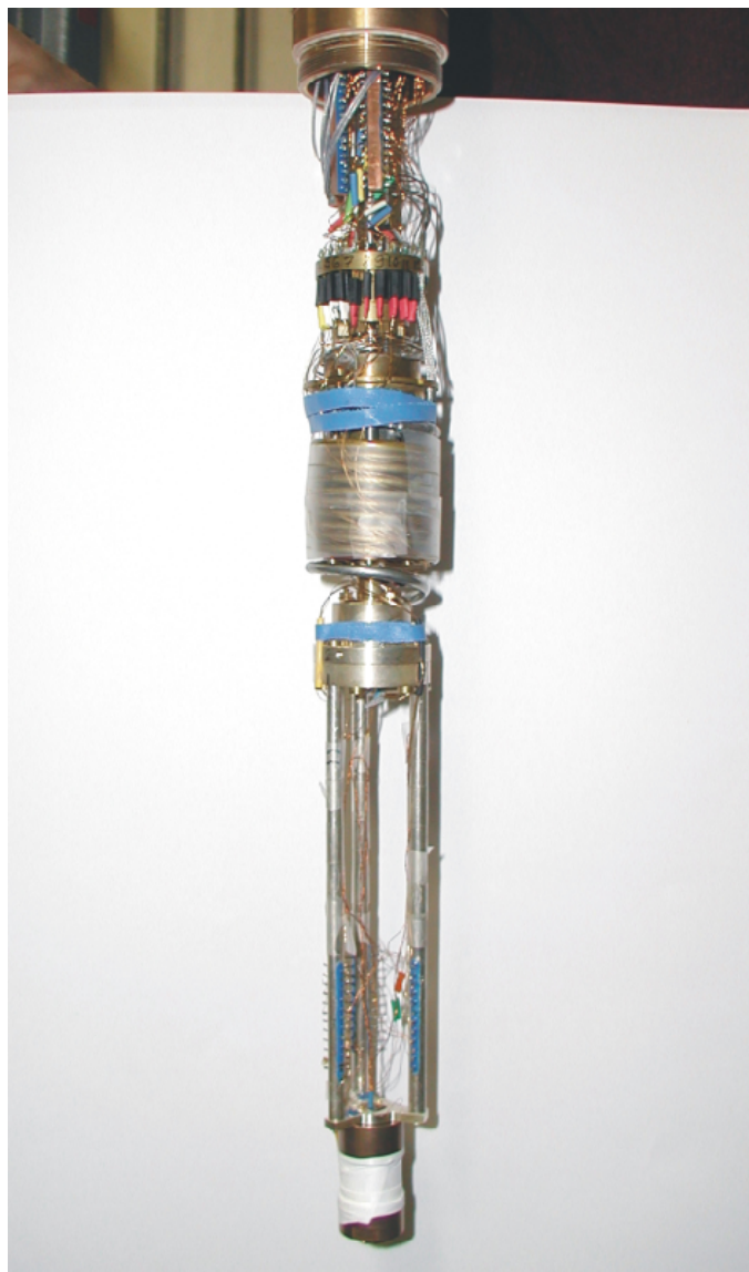
Figure 6.5: Inner (vacuum) part of the dilution refrigerator. The pressure cell is connected via silver rods to the mixing chamber.
