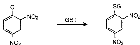
Figure 3. Conjugation of the standard substrate CDNB, (1-chloro-2,4-dinitrobenzene) to glutathione. The assay conditions are easy to meet and measurement of conjugate absorption at 340 nm in a spectrophotometer provides fast success even for beginners in enzymology, however, the substrate does not cover all glutathione S-transferases.
