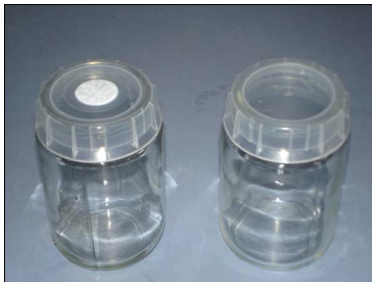
Figure 5. Baby food culture jars covered with Magenta B-CAP with filter (left) or without filter (right).
