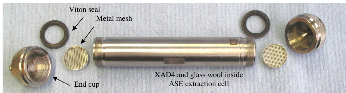
Figure 3.3. Adsorbent cartridge based on ASE extraction cell
