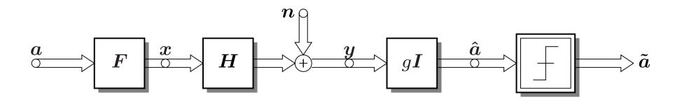
Principle: "predistortion" with  $F \in \mathbb{C}^{N_T \times N_R}$ : channel acts as equalizer correction of amplitude with scalar estimator  $g \in \mathbb{C}$  $\Rightarrow$  joint optimization
