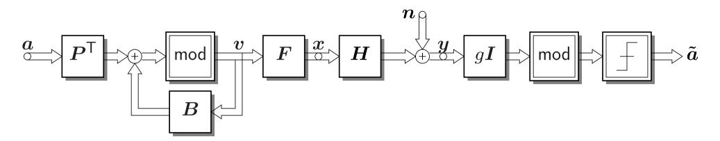
Principle:use already precoded symbols for interference reductionFeedback Filter:for realizability: lower triangular and zero main diagonal
