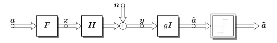
Criterion: minimization of mean square error with complete interference suppression
