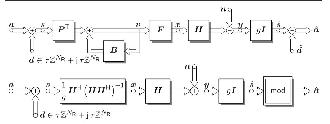
Principle: use ambiguity due to modulo operator at receiver for transmit power minimization
