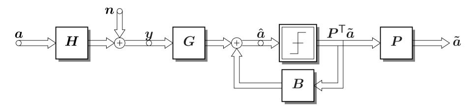
Principle: use already quantized symbols for interference reduction
