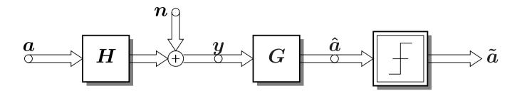
Principle: split into linear estimator  $G \in \mathbb{C}^{N_T \times N_R}$  and symbol-by-symbol quantizer
