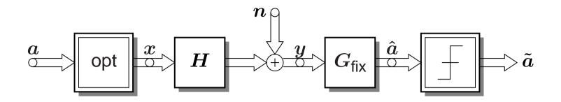
Principle: minimization of bit error probability by appropriate choice of transmit signal for given transmit power
