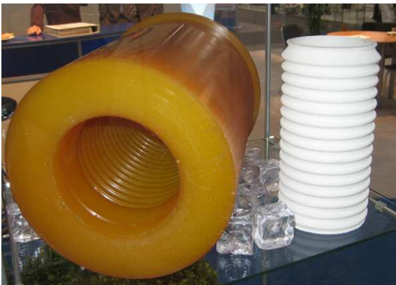
(a) Specimen made of \text{Al}_2\text{O}_3 together with its rubber mold
