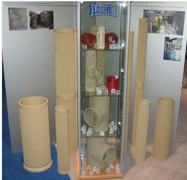
Figure 1.3: Chamotte tubes produced applying cold isostatic pressing by the German company Schiedel with Loomis presses (Ceramitec trade fair in Munich 2006)
