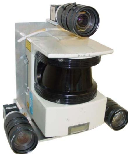
*Figure 3.1: TRIVIS - A three-camera system attached to a laser scanner*
