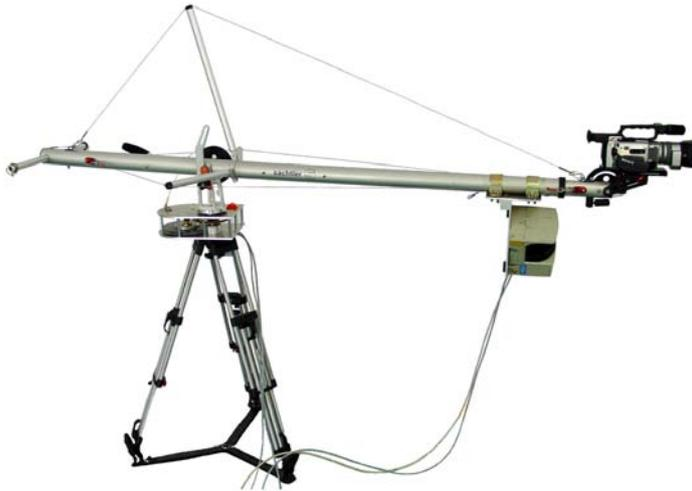
Figure A.3: Camera crane for the acquisition of concentric mosaics.
