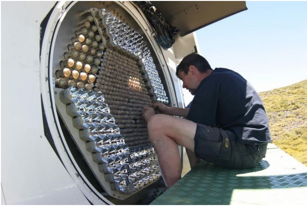
Figure 4.15: Photograph of the camera of the MAGIC telescope with opened lids, while the Winston cones are being installed. The inner part of the camera consists of 397 PMTs of 1" that are surrounded by 180 PMTs of 1.5" diameter.
