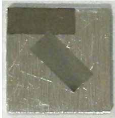
Figure 4.3: Al-sample with 5 mm wide W-strips. The size of the sample is 20 \times 20 mm.
