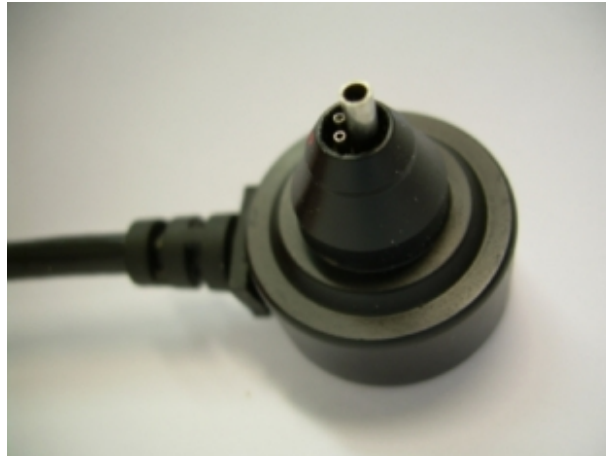
Figure 3.2: DPOAE ear probe (Etymotic ER-10C)
