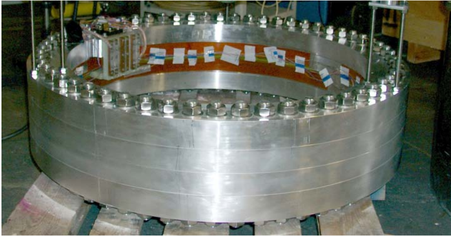
Figure 8.2: Two test coils similar to the outer storage coils of PENELOPE.
