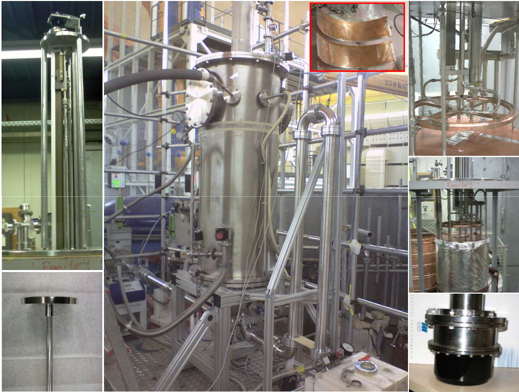
Figure 5.5: (Left top) Absorber cooling and drive system in 2007 with bellows - (left bottom) UCN storage valve V2 - (middle) AbEx installed at the experiment platform at ILL - (right top and middle) absorber support wheel with cooling pipes - (right bottom) ^3\text{He} UCN detector. Two copper blades with PE foil are shown in the red inlay.
