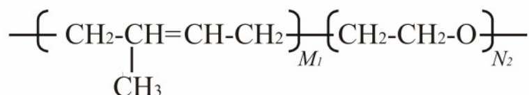
Figure 1.5 Structure of the poly(isoprene- b -ethyleneoxide) (PI- b -PEO) diblock copolymer. Symbol M_1 and N_2 represent the degree of polymerization of PI and PEO monomer, respectively.
