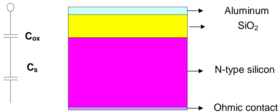
Figure 2.7 Schematic profile of a MOS capacitance (right), the equivalent circuit diagram consists of an oxide capacitance and a capacitance from the depleted layer (left).
