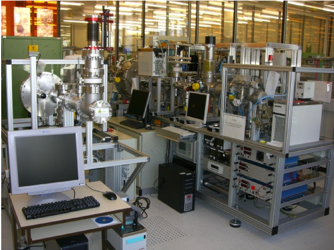
Figure 5.2 CaliFa setup in Semiconductor Labor Munich, which can provide X-ray irradiation with energy of about 17 keV.
