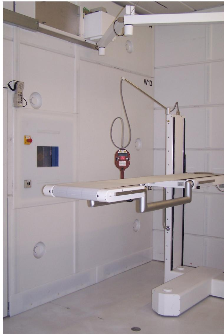
Figure 3.4: *View of the patient treatment couch; on the left, the beam exit window can be seen as well as the wooden hand panel for the couch in the centre.*
