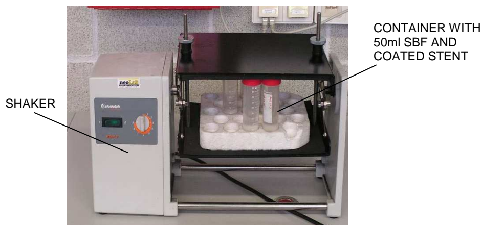
Fig. 6.13: Shaker for drug release test. To protect rapamycin from degradation in the light and to simulate bodily conditions the shaker was placed inside an incubator.
