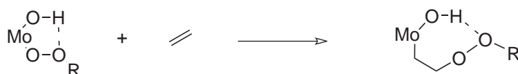
Scheme 2.15. The olefin coordination to the metal and the formation of the first C-O bond 98
