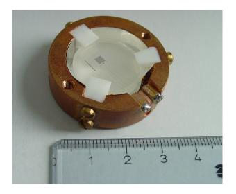
Figure 4.13: Picture of the phonon detector. The absorber is a  $CaWO_4$  cylindrical crystal of 20 mm diameter and 5 mm height. The TES evaporated onto the crystal is highly elaborate (see text). The detector is enclosed in a copper holder. On the inner side of the holder a reflecting foil is placed for the collection of the scintillation light [47].
