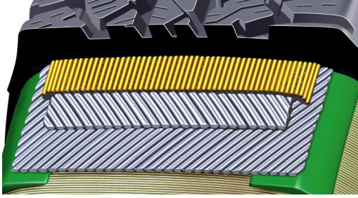
Figure 2.3: Cord-belt of a tire (courtesy of the Bridgestone Corporation)
