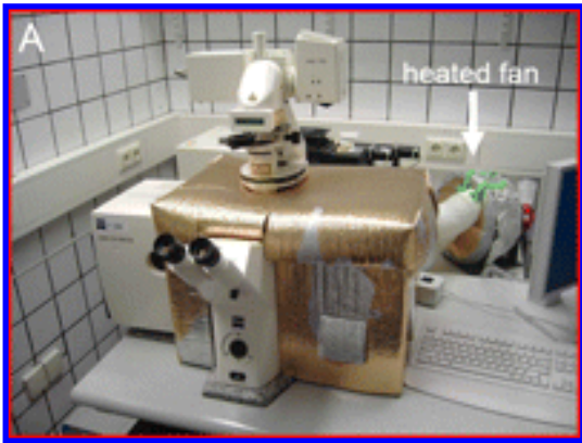
Figure 1. A Zeiss LSM 510 confocal microscope with a custom-fit incubation chamber. Cardboard covered with insulating foil was used to construct a custom-fit chamber around the microscope stage.
