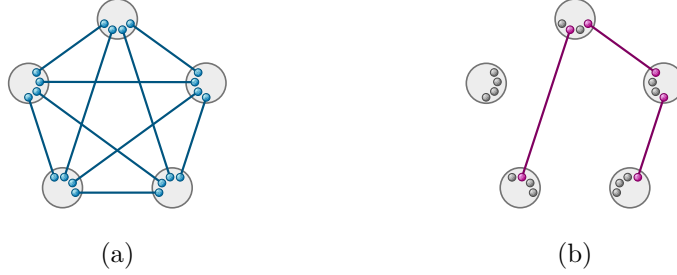
Figure 3.2: An example of a quantum random graph on five nodes. (a) Each node is in possession of four qubits which are entangled with the corresponding qubits at the other nodes. All the connections are given by the non-maximally entangled state |\varphi\rangle . (b) The quantum links can be converted into Bell pairs with probability p = 2\varphi_1 (here, p = 0.25 ). This strategy mimics the behavior of classical random graphs.
