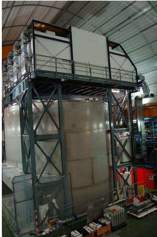
Figure 5.3.: Photo of the GERDA experiment taken in early summer 2009. The watertank inside the superstructure and the clean room on top can be seen.
