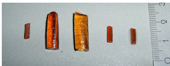
Figure 3.2.: Swelling of cross-linked PAN sticks in various solvents. From left to right: dry PAN-polymer stick of the first generation with 2.4 mm diameter and identical sticks after 5 days in DMSO, DMF, methanol and chloroform. [96]
