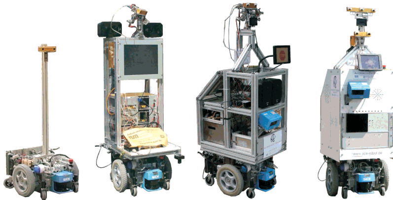
Fig. A.1: Development of ACE over the time, from basic platform to complete system.
