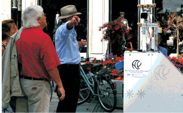
Fig. 2.3: ACE following the pointing gesture of a passer-by with its camera head.
