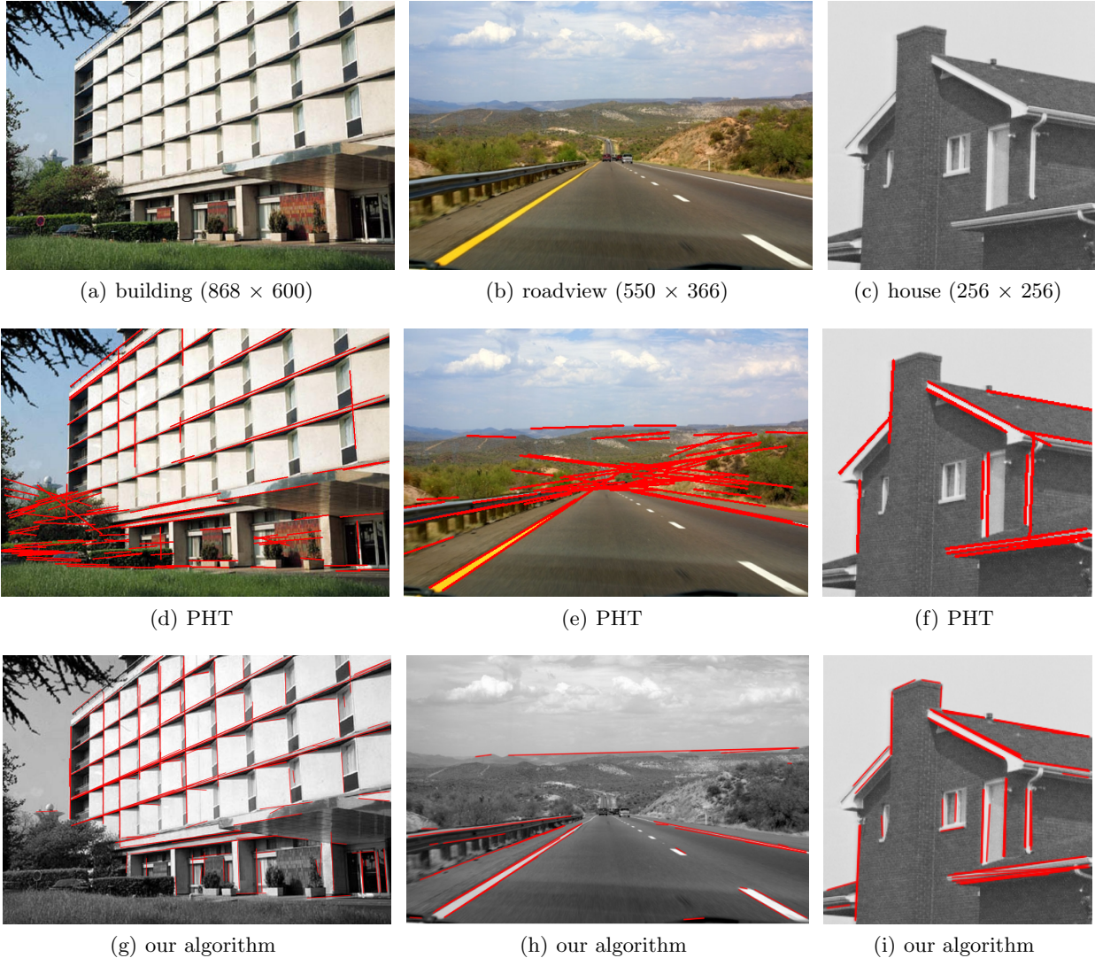
Figure 3. Example Input images a)-c), and their resulting Output of the Probabilistic Hough Transform (PHT) d)-f), and of the method proposed in this paper g)-i) .
