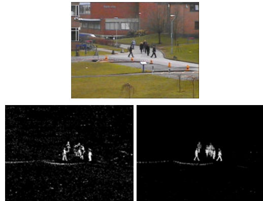
Figure 4: a) Input image. b) GMM based foreground segmentation c) Output of the proposed method.
