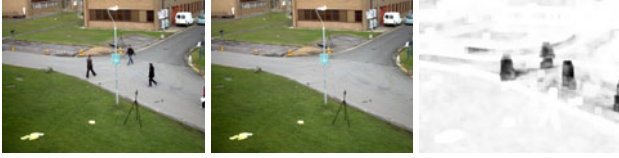
Figure 1: a) Input image. b) Reference image. c) NCC-based probability image between the reference image and the input image.
