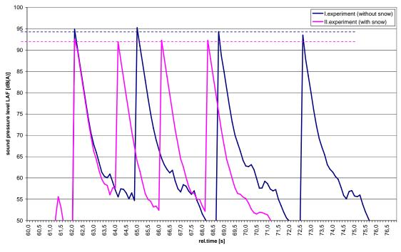
Figure 3: Comparison of the A- and Fast-weighted sound pressure level
