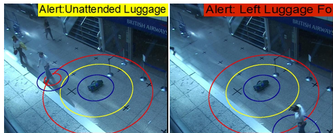
Fig. 14. A sample from S08. First the person leaves the 3m radius. After 25s an alert will be set
