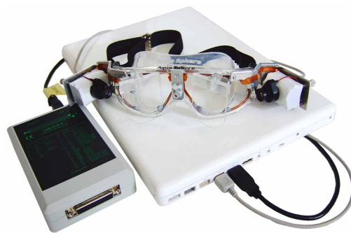
Figure 2: EyeSeeCam head-mounted mobile eye tracking system.
