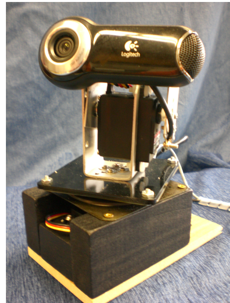
Fig. 1. The camera is mounted flexible in order to track the human's face. Head gestures are estimated from the acquired images.
