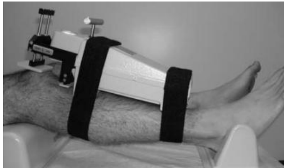
Figure 17: The KT 1000 Device to measure the femoro tibial translation. The punch with the handle applies force against the tibia, on a scale the examiner can read the translation in mm.
