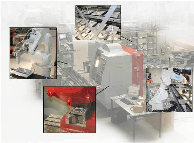
Figure 4: The hardware setup used for experimentation, showing storage, transport, robot and machining components.
