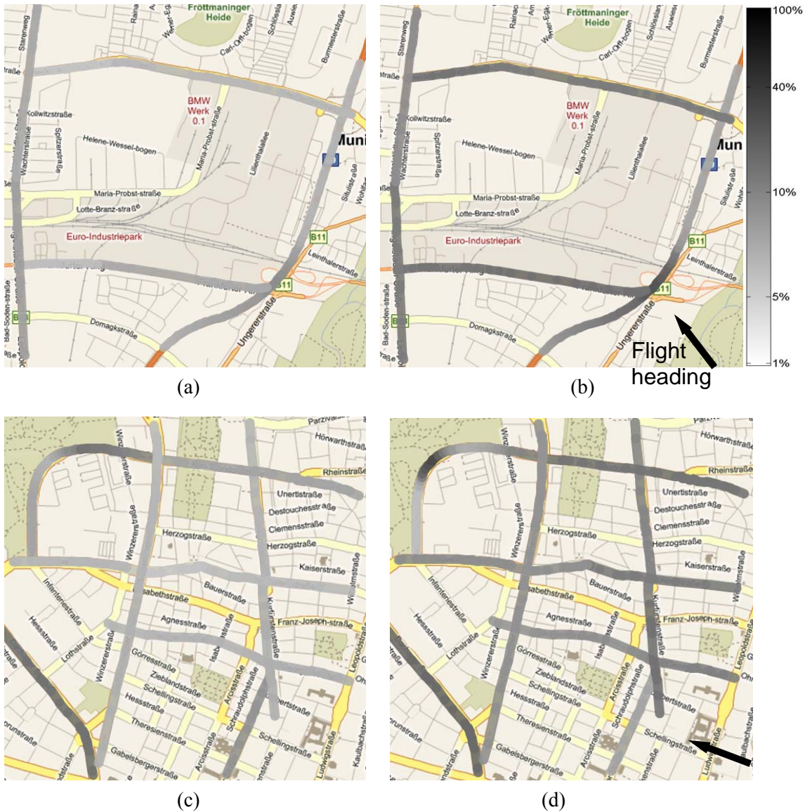
Figure 54: Simulation of standard deviation of velocity estimates \sigma_v on two road networks north of Munich using the velocity estimation schemes: (a) and (b) show the estimation accuracy for the first road network in % of the absolute velocity using the first and second schemes, respectively, (c) and (d) show the estimation accuracy for the second road network in % of the absolute velocity using the first and the second scheme, respectively
