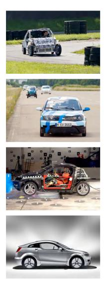
Visio.M BS1: Drivable tubular frame for the testing of vehicle components
